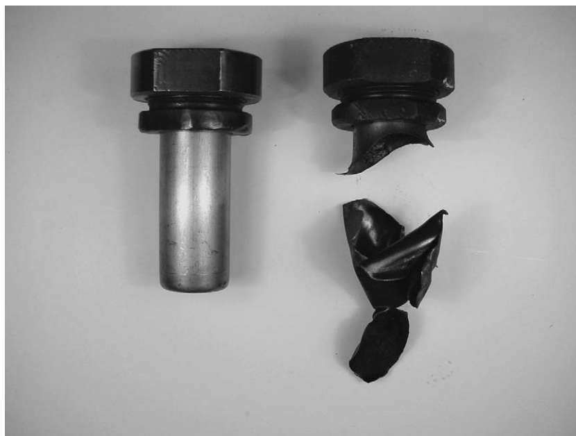
Fig. 10. TBTU, Koenen test at 2.0 mm.
