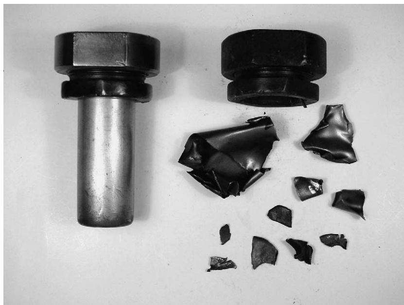
Fig. 3. HOBt, dry, Koenen test at 10.0 mm.
