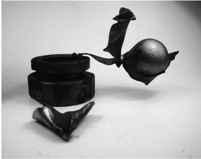
Fig. 4. HOBt with 44% water, Koenen test at 2.0 mm.
